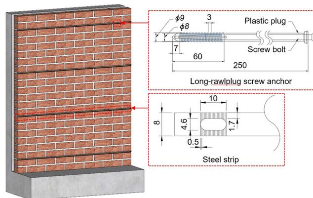
Fig. 1 Schematic of long-rawlplug screw anchor and steel strip
